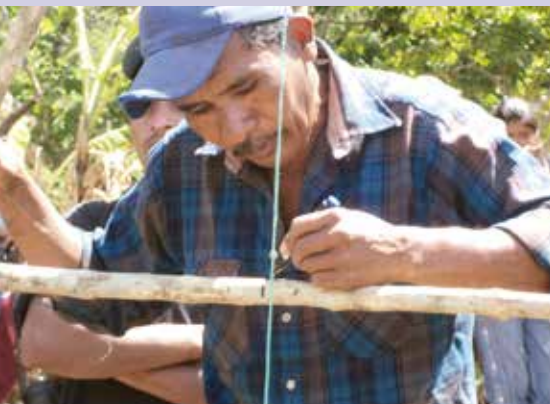
Jose Ramón Rivera calibrating an A-frame level in the Agroecological Coffee Field School in the community of La Fuente. (Photo: Nicaraguan Red Cross)
